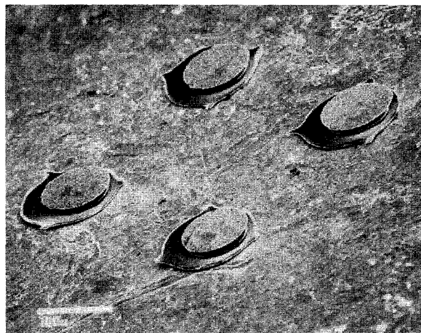
Figure 1. Web quad chip design allows four mesas to be thermocompression-bonded directly to the diamond heat spreader.
